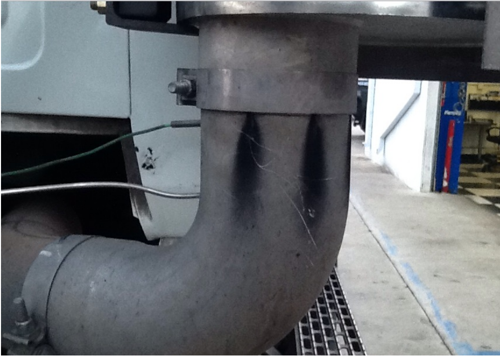
Installed SEAL CLAMPS in place of all leaking AccuSeal (TM) Clamps (and cleaned all soot off truck)
